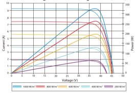
Excellent performance under weak light conditions: at an irradiation intensity of 200 W/m<sup>2</sup> (AM 1.5, 25 °C), **96.5%** or higher of the STC efficiency (1000 W/m<sup>2</sup>) is achieved
