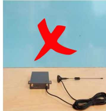
3G/4G Antenna is horizontal
