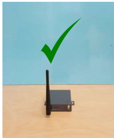
WiFi antenna is mounted upright
