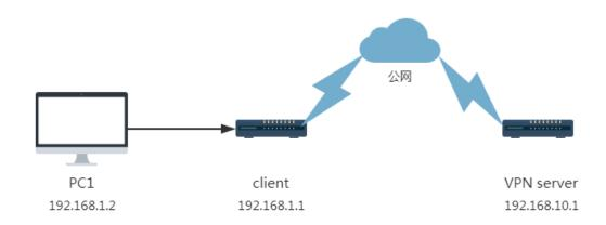
Select "Redirect Internet traffic", after Router connects to 4G network, PPTP Client will connect to PPTP Server and get the IP and Gateway. And Router can ping the Gateway of PPTP Server
