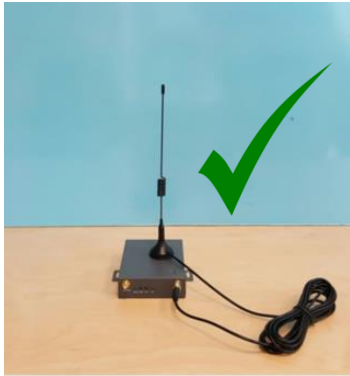
3G/4G Antenna mounted upright on metal surface
