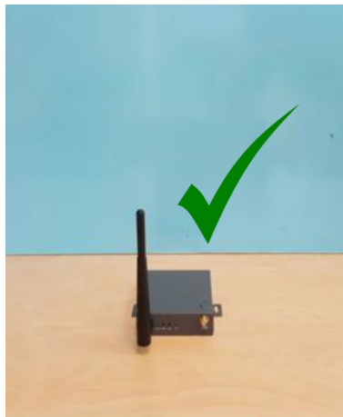
WiFi antenna is mounted upright
