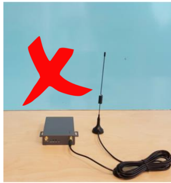
3G/4G Antenna mounted upright on non-metal surface
