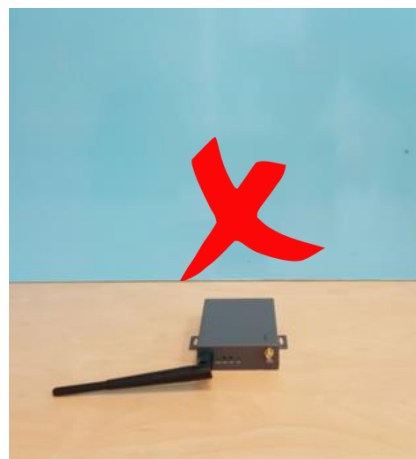
WiFi antenna is mounted horizontally
